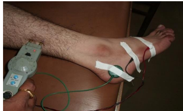
Fig 1: Electrode placement for Sural Nerve Sensory Nerve Conduction study at 14 cm distance.
